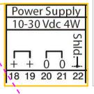
Note: Pin 22 - Shld. - is the chassis ground
